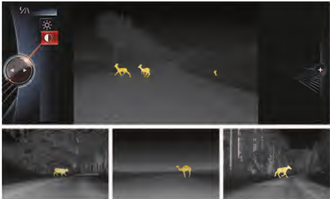
BMW 5 Series LCI Night Vision camera image for identified animals on the central information display
